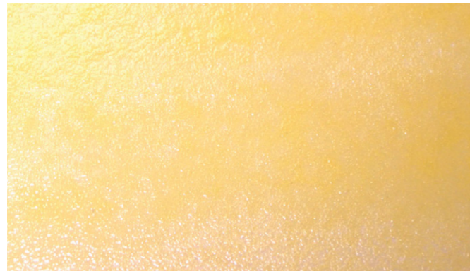
COVERAGE TOO HEAVY
