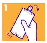
Shake the cartridge vigorously for 60 seconds, then stand cartridge upright for at least 1 minute allowing any bubbles to rise to the top.
