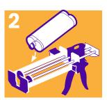
Insert cartridge into the dispenser. Make sure it is properly positioned with the shoulder of the cartridge flush with the front/top bracket of the dispenser. Point upward at
